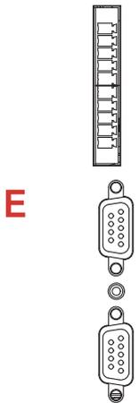
**Parallel ports:** The parallel ports will enable the connection of up to four units in parallel by using the optional cable kit (one for each unit).
