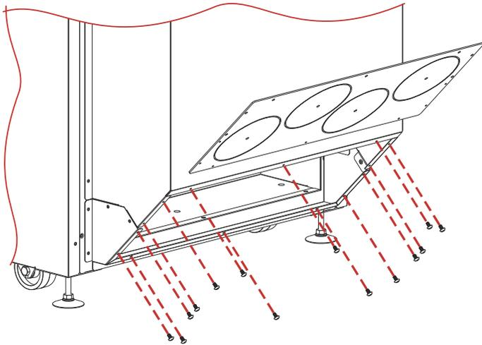
Remove the terminal block cover aluminum panel.
