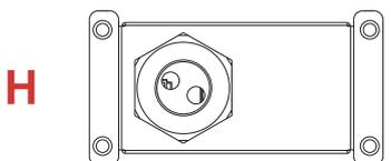
**External signals cover:** remove this cover to access the external signal connectors.
