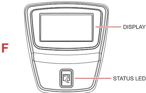
**Touch screen display and led indicator:** Through the 5" touch panel display the user can monitor the system parameter and configure the UPS. The Riello logo backlight color indicates the system status. Refer to User Manual for further information.
