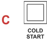
**Cold start button:** This button allows the user to turn the UPS on from battery, even without the mains present. Refer to User Manual for further information.
