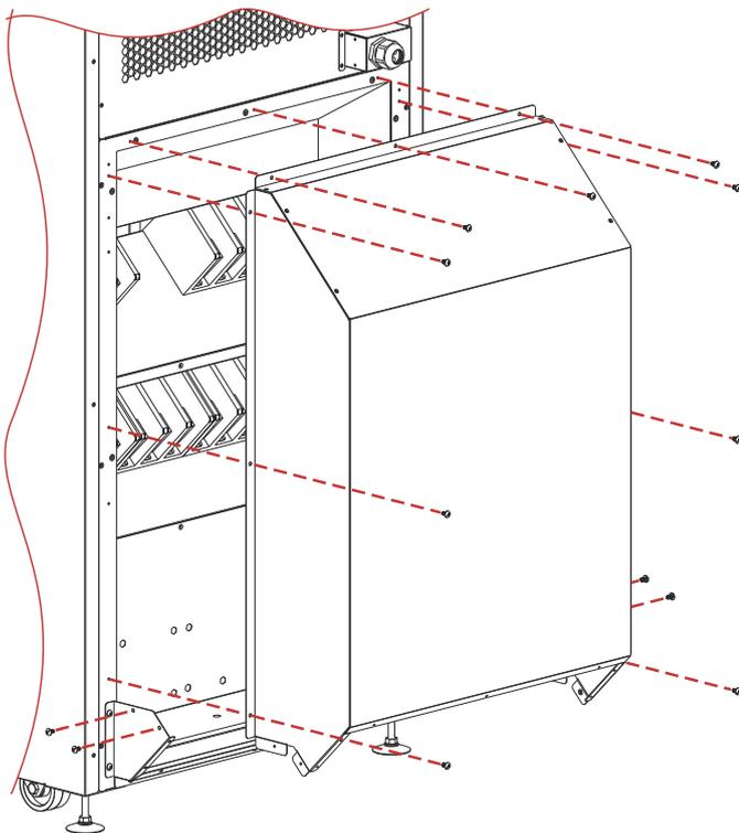
Remove the bigger part of the cover to access the terminal blocks.
