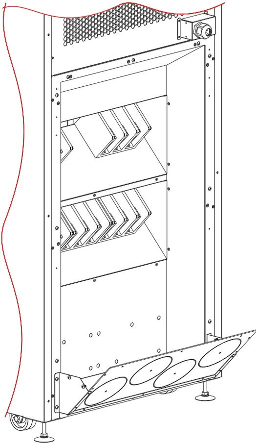
Put the aluminum plate in place and fasten it with the provided screws, after passing the power cables through it.
