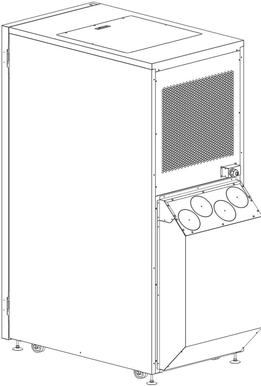
If top cable entry is required by the installation, the rear terminal cover can be rotated by 180 degrees to enable the wiring to exit upward.
