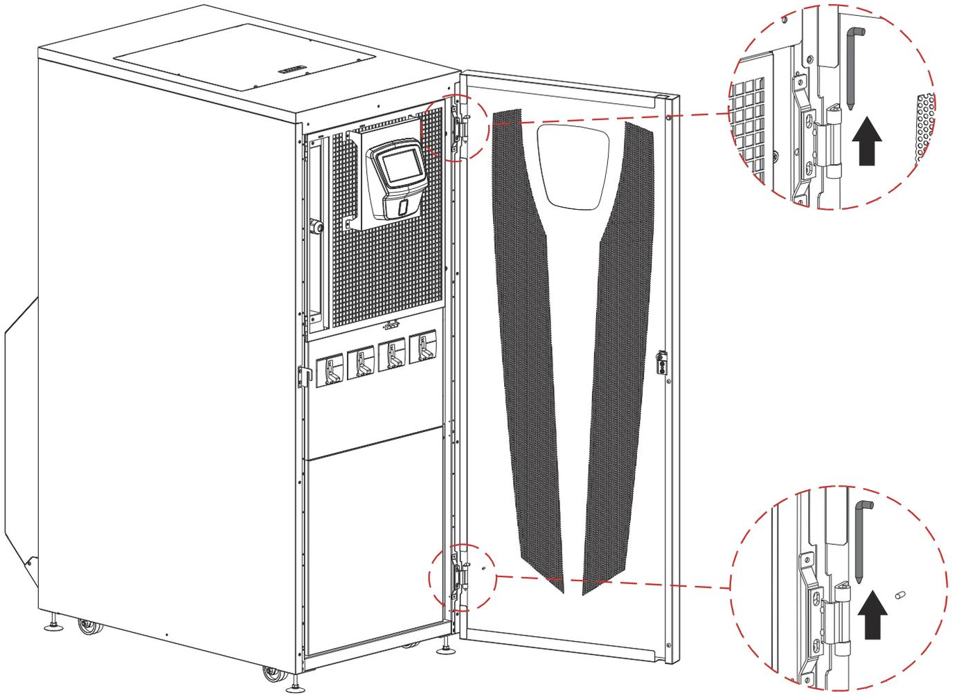
To remove the door, first remove the PE connection on the bottom part of the door. Then pull out the pins from the top and bottom hinges and take off the door.
