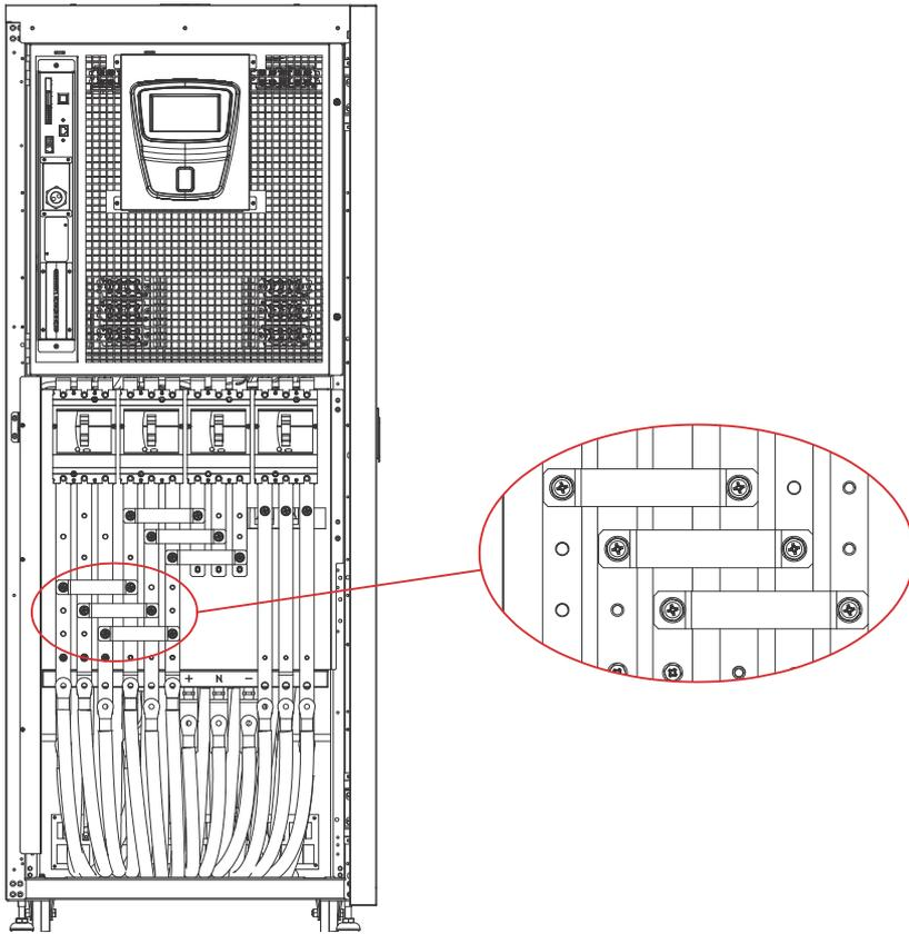
To access the bridges, it is necessary to remove the front breaker covers below the door.
