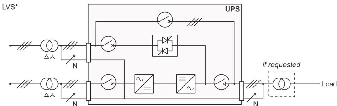
**UPS without any variation in neutral condition and with separate bypass input**
