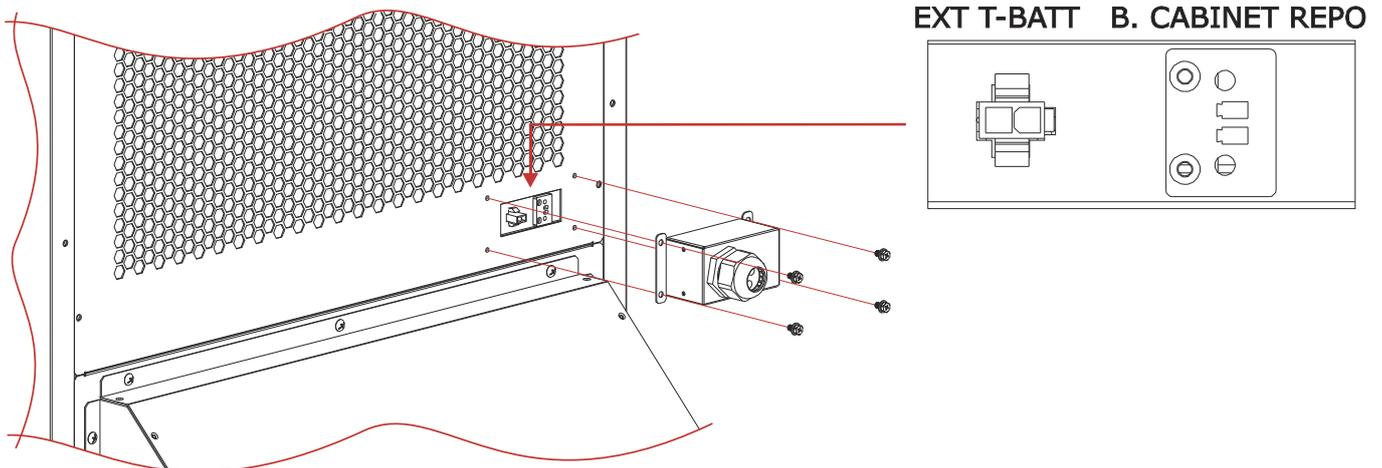
On the UPS rear, just above the terminal block cover, there are two signal connectors, enclosed in a metal cover:
