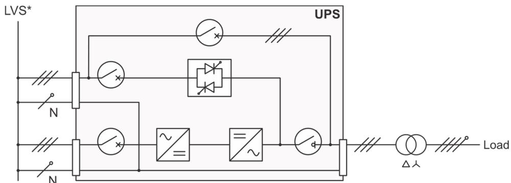
**UPS with galvanic isolation and with separate bypass input**
