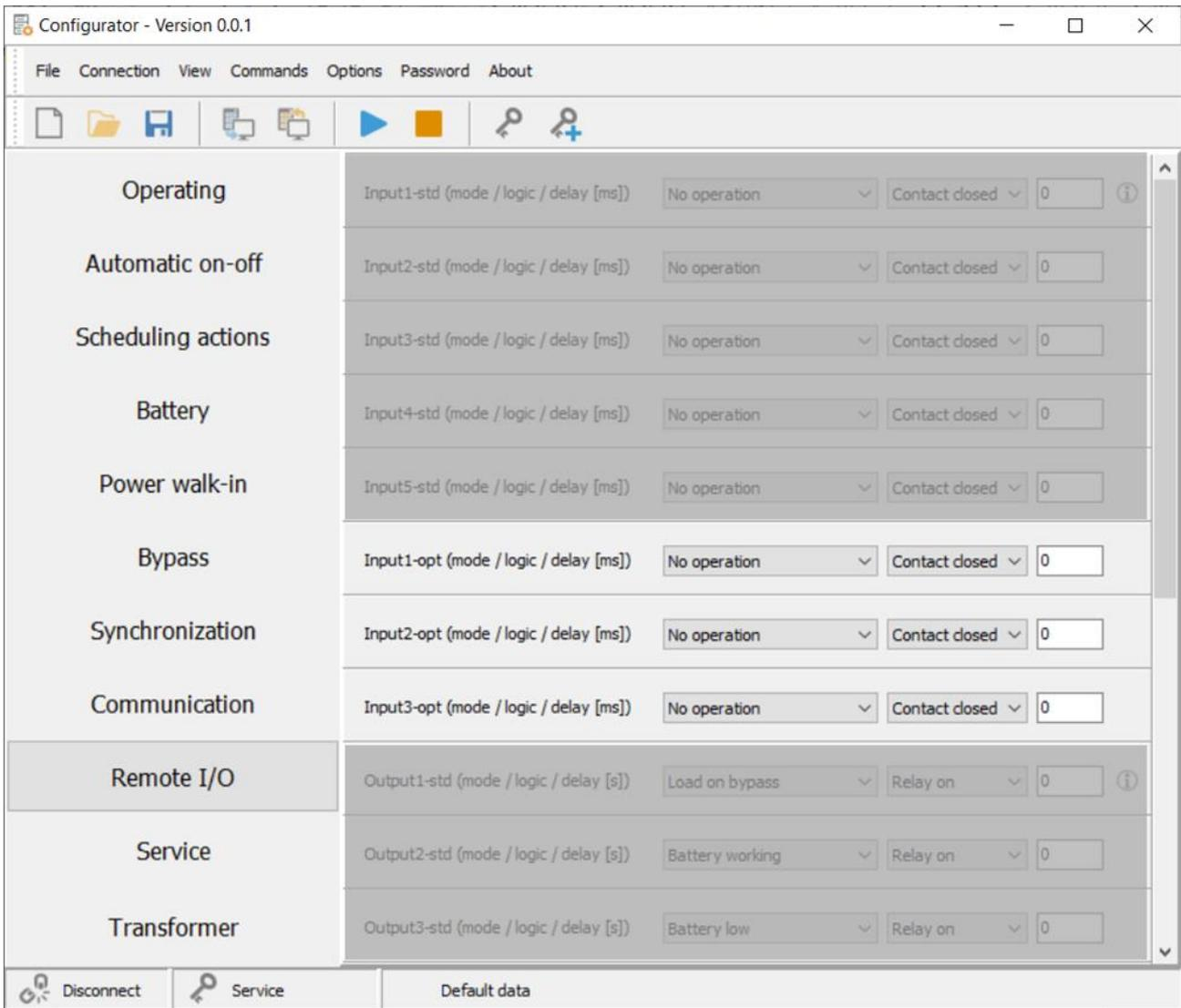
**i** For each input can be selected: the associated function (Mode) and the operating logic of the contact (Logic).
