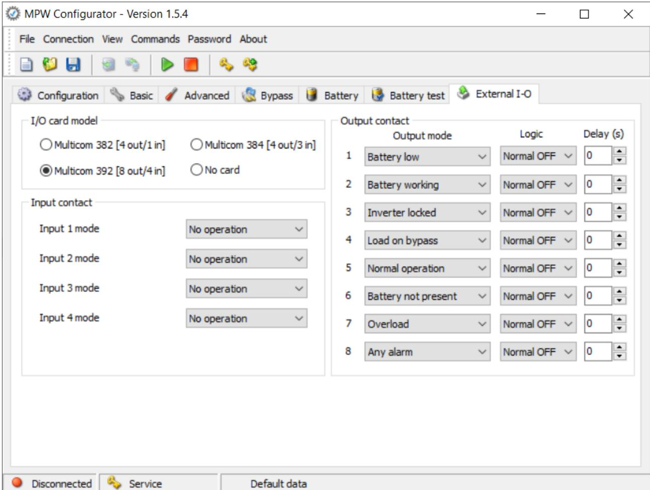
**i** For each input can be selected: the associated function (Input mode).
