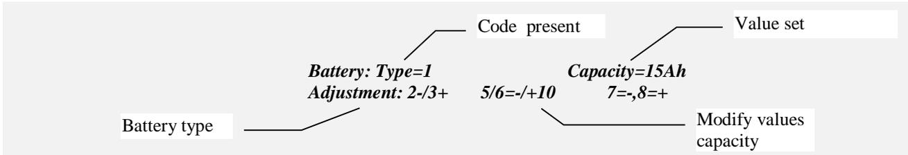
On initial installation the rated capacity value of the connected battery must be inserted; this value is usually printed on the battery container.
