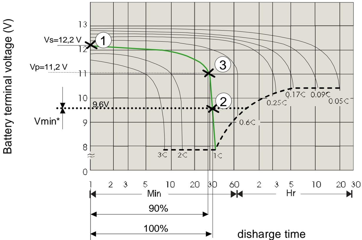
The three values, Vs, Vmin and Vp, are obtained from the discharge characteristic curve, supplied from manufacturer, relating to the **battery discharge regime** 1C has been determined:
