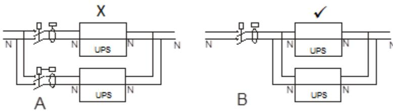
It is recommended that a Ground Fault Interrupter (GFI) device is implemented for safety. In order to avoid unnecessary interventions, versions with several parallel-connected devices must have a single GFI device inserted at the input of the whole system, as shown in figure B.
