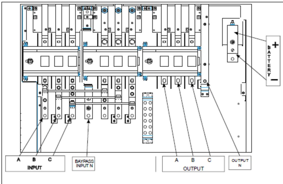
Note: For the Input, Output and Battery connections, follow the order from the top to bottom, or right to left, as described in the boxes. The label marked “N” present on the terminal identifies the neutral terminal.
