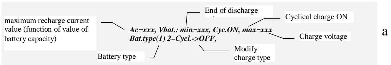
Select type 0 and then press key 4 to modify the voltage values reset by keys 3,4 and 7,8.
