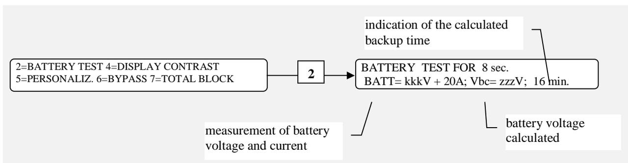
This activates the cycle to check the state of efficiency of the battery, which lasts 8 seconds. Press key 8 to interrupt the test and return to the basic menu before this time has elapsed.
