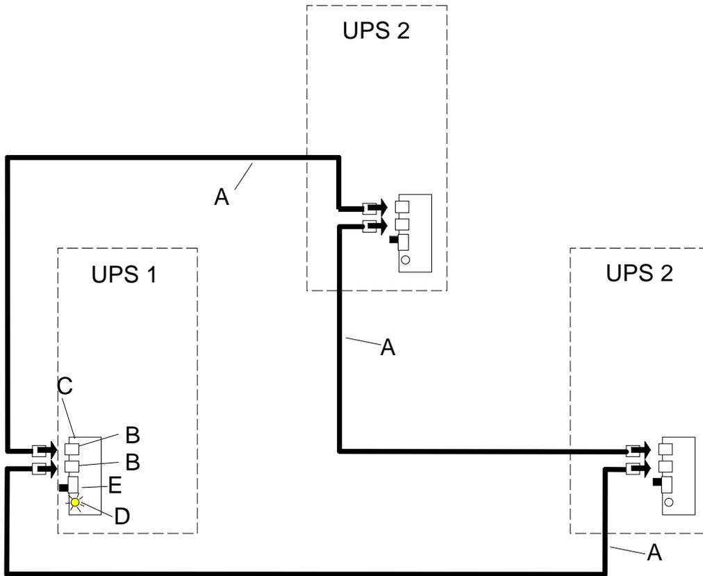
To add other parallel UPS's, a "UPS PARALLEL CABLE" must be added for each new UPS connected.
