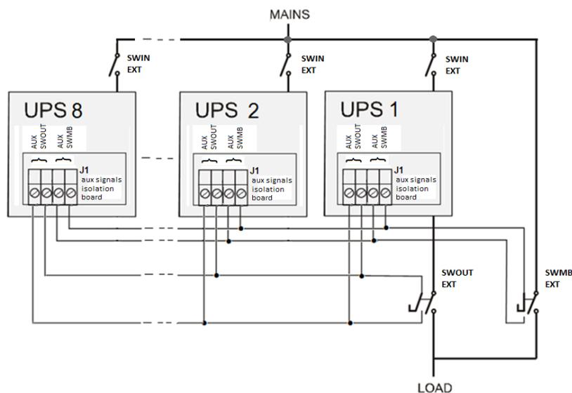
The auxiliary contacts of SWOUT EXT and SWMB EXT must be connected to terminal J1 on aux signals isolation board. The purpose of this board is to isolate the internal circuits of UPS, so that, in case of parallel of UPS, one auxiliary contact of an external switch is sufficient to be acquired by all the UPS in parallel.
