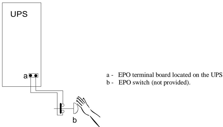
On the UPS, the jumper on the EPO terminals must be removed, and the wires from the auxiliary contact of the pushbutton must be connected in place of the jumper.
