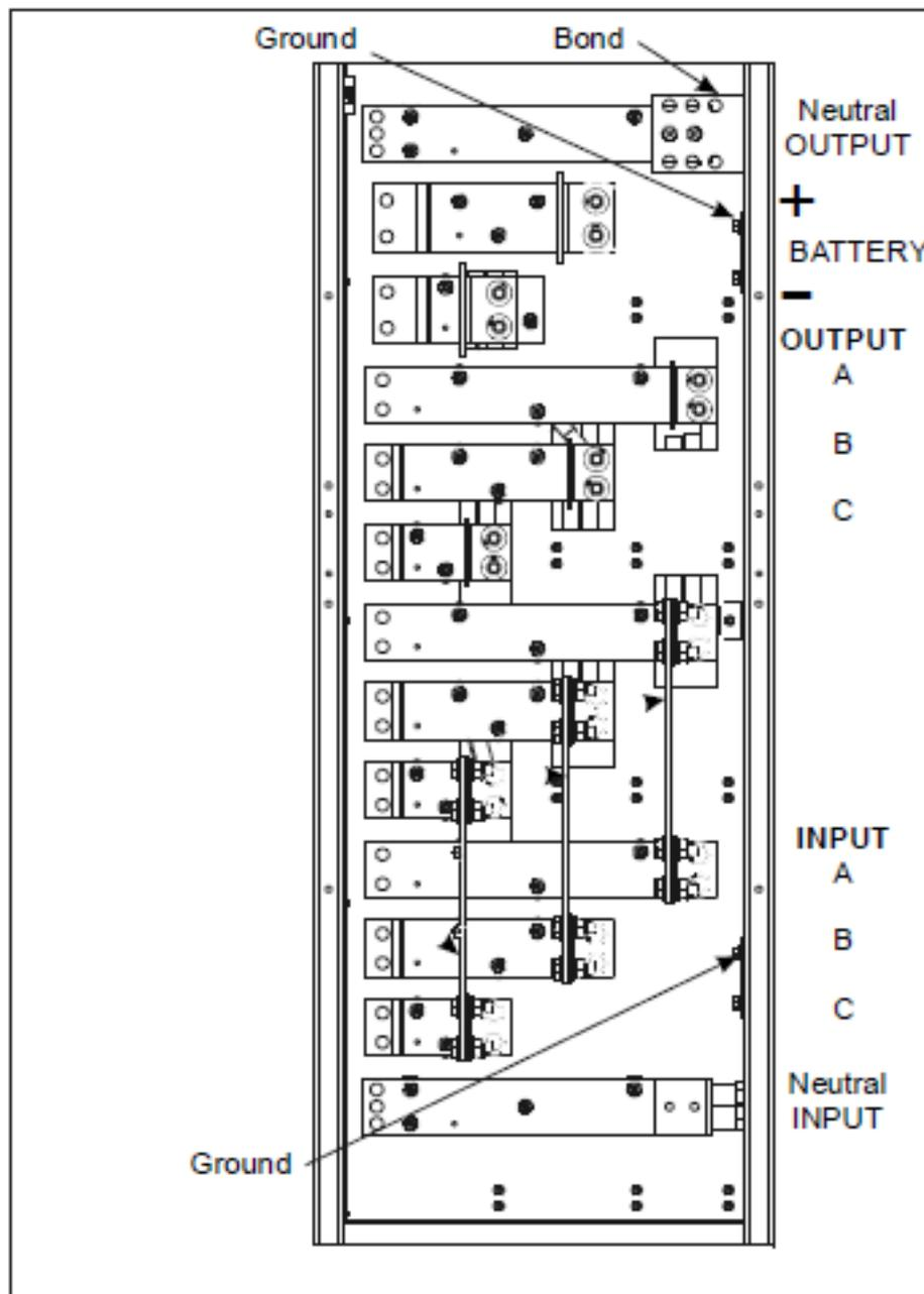
Note: For the Input, Output and Battery connections, follow the order from the top to bottom, or right to left, as described in the boxes. The label marked “N” present on the terminal identifies the neutral terminal.
