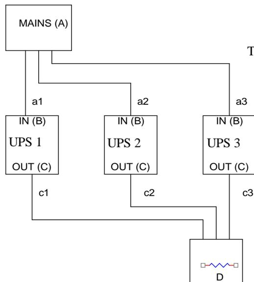
The figure shows an example of three units connected in parallel.
